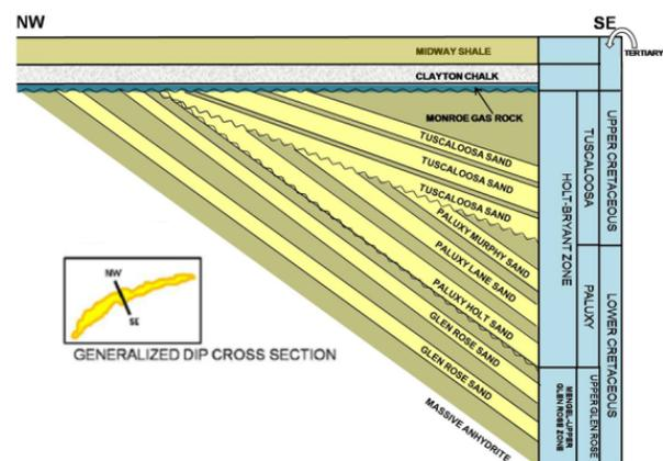
Figure 2: Northwest to southeast PP seismic cross-section showing the trap of the reservoir. The main reservoir is composed of Paluxy and Tuscaloosa sandstones. The top seal corresponds to the Midway Shale. Note that the pinch out is located from southwest to northeast (modified from Denbury Resources Inc).
