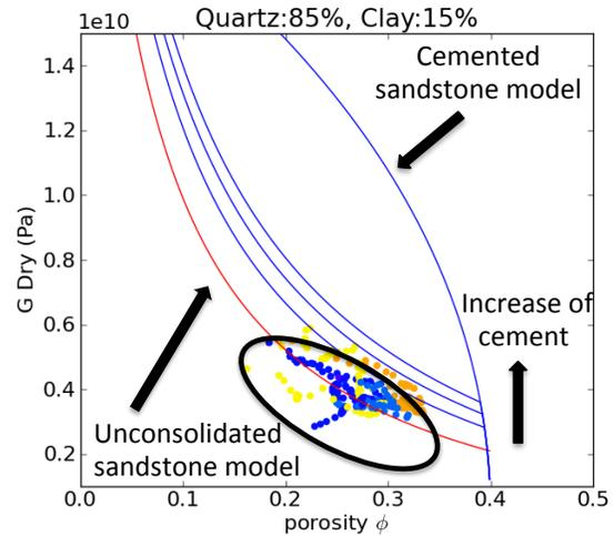
Figure 3: Rock physics model calibration for the Paluxy and lower Tuscaloosa facies. The scatter points represent the shear modulus values obtained from the well logs. Note that the values fit the unconsolidated sandstone model.
